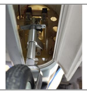
11. The tail retract installed to the fuselage and the wires inside the fuselage.
