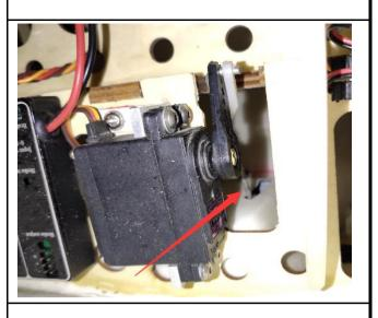
5. Assemble the main retracts and gear cover parts to the retract mount with screws.
