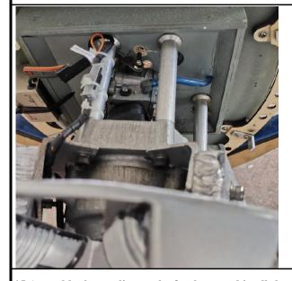
15.Assemble the cowling to the fuselage, and instll the propeller and spinner to the engine .
