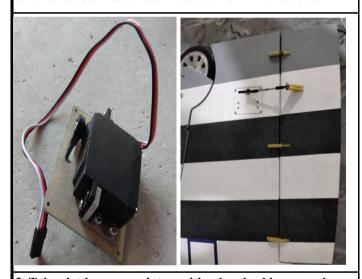
3. Trim slot in appropriate position in wheel house and connect the gear door to the gear door servo, see the pictures.
