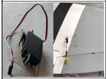
2. Assemble the flap on the outer wing. Prepare the servos for flaps, trim slots to appropriate position in the wing and flaps, apply instand type AB glue to the slots in the flaps and horns. Connect the servo to the horn with screws.
