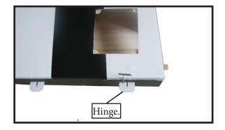
3) Slide the wing panel on the aileron until there is only a slight gap. The hinge is now centered on the wing panel and aileron. Remove the T-pins and snug the aileron against the wing panel. A gap of 1/64" or less should be maintained between the wing panel and aileron.
