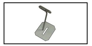
2) Remove each hinge from the wing panel and aileron and place a T-pin in the center of each hinge. Slide each hinge into the wing panel until the T-pin is snug against the wing panel. This will help ensure an equal amount of hinge is on either side of the hinge line when the aileron is mounted to the aileron.
