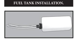
You should mark which tube is the vent and which is the fuel pickup when you attach fuel tubing to the tubes in the stopper. Once the tank is installed inside the fuselage, it may be difficult to determine which is which. 7) Slide the fuel tank into the fuselage. Guide the lines from the tank through the hole in the firewall.
