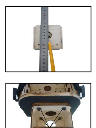
4) Attach the motor to the front of the electric motor box using four 4mm blind nut, four M3x15mm hex head bolts to secure the motor. Please see picture shown.
