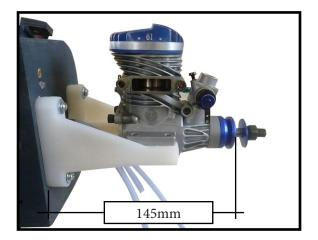
2) Use a pin drill and 4mm drill bit to drill a small indentation in the mount for the engine mounting screw.
