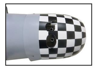
2) While keeping the back edge of the cowl flush with the marks, align the front of the cowl with the crankshaft of the engine. The front of the cowl should be positioned so the crankshaft is in **nearly** the middle of the cowl opening. Hold the cowl firmly in place using pieces of masking tape.
