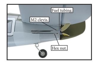
Insert fuel tank onto the wings.
