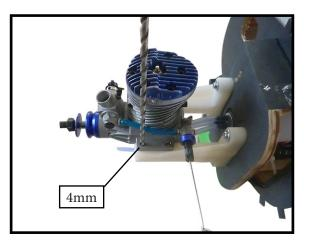
3) Use a drill to drill the four holes in the engine mount rails.
