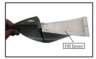
2) While holding the vertical stabilizer firmly in place, use a pen and draw a line on each side of the vertical stabilizer where it meets the top of the fuselage.
