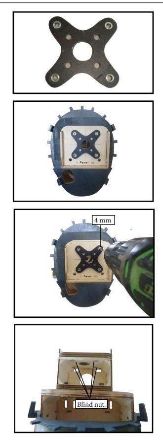
5) Attach the motor to the front of the electric motor box using four 4mm blind nut, four M3x15mm hex head bolts to secure the motor. Please see picture shown.
