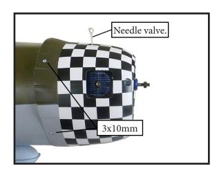
3) Install the muffler and muffler extension onto the engine and make the cutout in the cowl for muffler clearance. Connect the fuel and pressure lines to the carburetor, muffler and fuel filler valve. Secure the cowl to fuselage using the M3x10mm screws.
