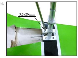
2) Install servo for Retractable landing gear.
