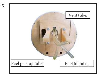
8) Connect the lines from the tank to the engine and muffl. Th vent line will connectto the muffl and the line from the clunk tothe carburetor.
