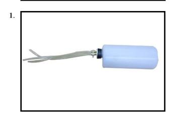
You should mark which tube is the vent and which is the fuel pickup when you attach fuel tubing to the tubes in the stopper. Once the tank is installed inside the fuselage, it may be diffilt to determine which is which.
