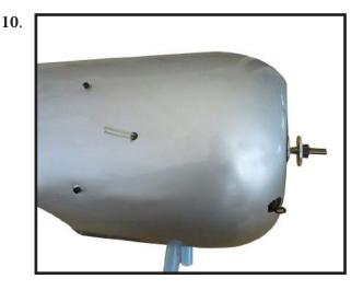
4) Install the muffl and muffl extension onto the engine and make the cutout in the cowl for muffl clearance. Connect the fuel and pressure lines to the carburetor, muffl and fuel filer valve. Secure the cowl to fuselage using the M3x10mm socket head screws.
