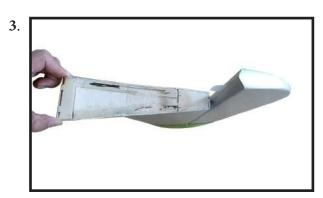
2) Slide the vertical stabilizer into the slot in the top of the fuselage. Th rear edge of the stabilizer should be flsh with the rear edge of the fuselage and the lower rudder hinge should engage the precut hinge slot in the lower fuselage. Th bottom edge of the stabilizer should also be fimly pushed against the top of the horizontal stabilizer.
