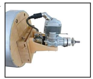
Blow through one of the lines to ensure the fuel lines have not become kinked inside the fuel tank compartment. Air should flw through easily.
