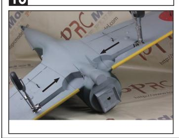
Assemble the inner gear doors to the fuselage with screws and epoxy, connect the horn on the inner gear door to the servo with push rod.
