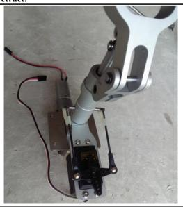
29. Assemble the nose retract to the fuselage with screws and assemble the back half nose gear door.
