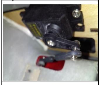
25.Connect the innner gear doors and the servos through the slot in the fuselage
