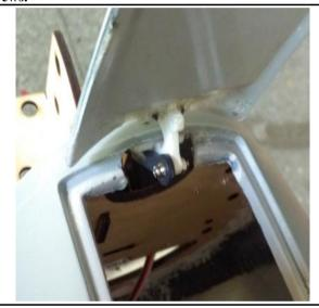
28. Assemble the nose landing gear and the servo to the nose retract.
