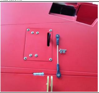
10. Connect the fiber horns to the servo arms with the linkage and lock each side with screws and nut.
