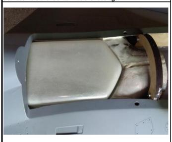
39. Assemble the engine and tail pipe to the fuselage with screws.
