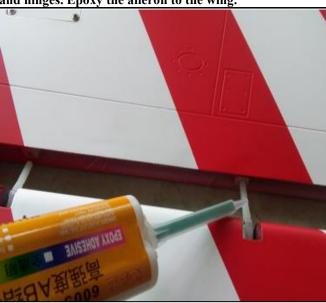
4. Apply AB glue to the slots in the ailerons, and assemble the horns into them.
