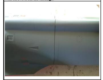
38. Assemble the fuel tank to the fuselage.
