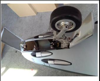
30. Connect the back half nose gear door to the landing gear with push rood and screws.
