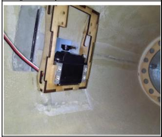
20. Connect the plastic horn in the belly brake to the servo arm with the linkage and lock each side with screws and locknuts.
