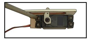
6) Apply 1-2 drops of thin C/A to each of the mounting tabs. Allow the C/A to cure without using accelerator.
