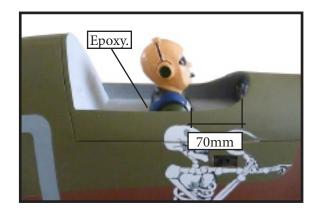
4) Position the canopy onto the fuselage. Trace around the canopy and onto the fuselage using a felt-tipped pen. Carefully cut and remove covering material from the fuselage where the canopy makes contact, exposing the bare wood. Then permanently glue the canopy in place with epoxy glue or special "canopy glue".
