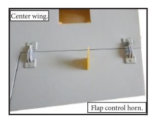
Then, fit the joiner wire into the flap of center wing as below pictures.
