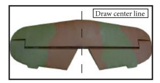
2) Using a modeling knife, carefully remove the covering at mounting slot of horizontal stabilizer ( both side of fuselage).
