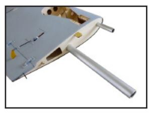
Slide the wing panel into position, guiding the extensions from the side wing into center wing.
