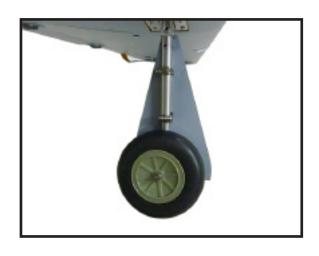
Slide the wheel on the axle, then secure it using the wheel collar.
