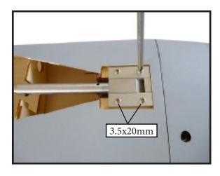
Install servo for wings gear.
