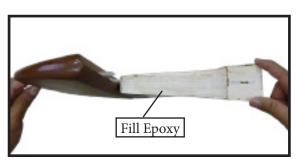
2) Slide the vertical stabilizer into the slot in the top of the fuselage. The rear edge of the stabilizer should be flush with the rear edge of the fuselage and the lower rudder hinge should engage the precut hinge slot in the lower fuselage. The bottom edge of the stabilizer should also be firmly pushed against the top of the horizontal stabilizer.
