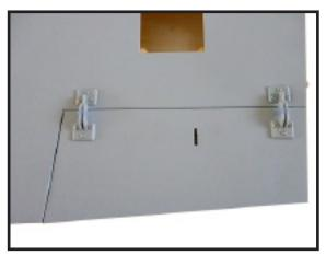
INSTALL FLAP CONTROL HORN FOR CENTER WING.
