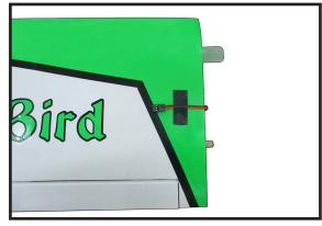
Reinstall the servo into the servo mount and secure the servo inplace using the wood screws provided with you radio system.
