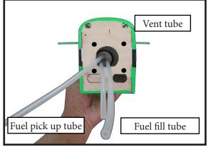
Connect the lines from the tank to the engine and muffler. The vent line will connect to the muffler and the line from the clunk tothe carburetor.
