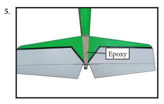
Slide the vertical stabilizer back inplace. Using a triangle, check to ensure that the vertical stabilizer is aligned 90° to the horizontal stabilizer.
