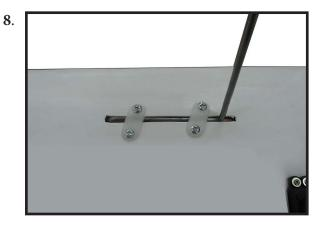
Reinstall the gear wire and install the straps using the four 3mm x 15mm wood screws. Tighten the screws completely to secure the gear wire in place.
