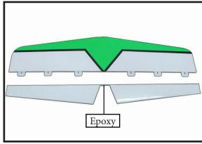
Glue the elevator hinges in place using the same techniques used to hing the ailerons.
