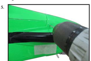
Install the muffler and muffler extension onto the engine and make the cutout in the cowl for muffler clearance. Connect the fuel and pressure lines to the carburetor, muffler and fuel filer valve. Secure the cowl to fuselage using the M3x10mm socket head screws. Putting a small length of silicon fuel tube under the head of the screw helps with vibration.
