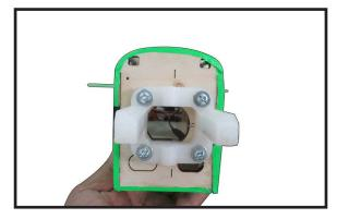
Position the engine with the drive washer (105mm) forward of the firewall as shown
