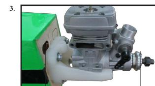
Use a pin drill and 3mm drill bit to drill a small indentation in the mount for the engine mounting screw.
