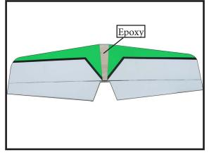
When you are sure that everything is aligned correctly, mix up a generous amount of 30 Minute Epoxy. Apply a thin layer to the top and bottom of the stabilizer mounting area and to the stabilizer mounting platform sides in the fuselage. Slide the stabilizer in place and realign. Double check all of your measurements once more before the epoxy cures. Hold the stabilizer in place with T-pins or masking tape and remove any excess epoxy using a paper towel and rubbing alcohol.
