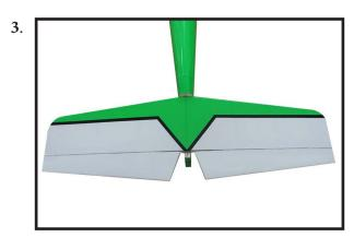
With the stabilizer held firmly in place, use a pen and draw lines onto the stabilizer where it and the fuselage sides meet. Do this on both the right and left sides and top and bottom of the stabilizer.
