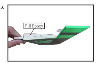
Slide the vertical stabilizer into the slot in the top of the fuselage. The rear edge of the stabilizer should be flush with the rear edge of the fuselage and the lower rudder hinge should engage the precut hinge slot in the lower fuselage. The bottom edge of the stabilizer should also be firmly pushed against the top of the horizontal stabilizer.
