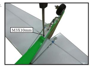
Adjust the wheel collar shown to set the height of the tailwheel wire. Then check to see if the long steering leg of the tailwheel wire is parallel to the bottom of the rudder. The wire may need to be tweaked slightly to make it parallel.
