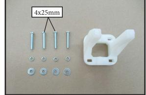
Use four 4x25mm head bolts and four 4mm washers to attach the engine mount rails to the firewall. Tighten the screws .Make sure to use threadlock on the screws to help prevent them from vibrating loose.
