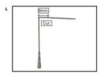
Make a 90-degree bend at the mark and cut off the excess wire leaving 8mm past the bend.
