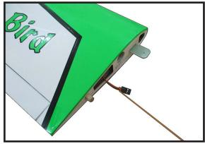
Tape the servo lead to the wing to prevent it from falling back into the wing.
