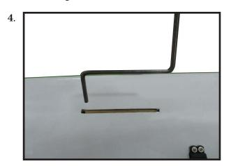
The landing gear wire is held in place using two nylon landing gear straps and four 3mm x 15mm wood screws.
