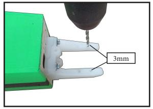
On the fie wall has the location for the throttle pusshrod tube (pre-drill).
