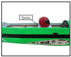
Position the canopy onto the fuselage. Trace around the canopy and onto the fuselage using a felt-tipped pen. Carefully cut and remove covering material from the fuselage where the canopy makes contact, exposing the bare wood. Then permanently glue the canopy in place with epoxy glue or special "canopy glue".
