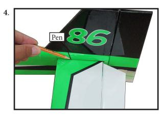
Remove the stabilizer. Using the lines you just drew as a guide, carefully remove the covering from between them using a modeling knife.
