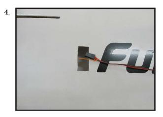
Attach servo lead to the aileron servo. Attach the string to the servo lead and carefully thread it though the wing. Once you have thread the lead throught the wing, remove the string so it can use for the other servo lead.
