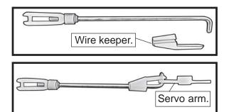
9) Connect the linkage as shown and secure the control wire with a wire keeper.
