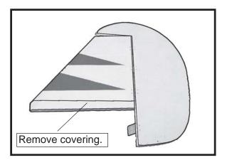
When cutting through the covering to remove it, cut with only enough pressure to only cut through the covering itself. Cutting into the balsa structure may weaken it.
