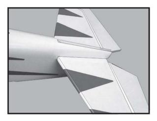
7) After the epoxy has fully cured, remove the masking tape or T-pins used to hold the stabilizer in place. Carefully inspect the glue joints. Use more epoxy to fill in any gaps that may exist that were not filled previously and clean up the excess using a paper towel and rubbing alcohol.
