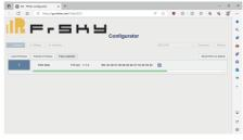
Step 4: Click the "Local Firmware" button and find Step 5: Click the tab "Flash selected" waiting for the completion of the flashing bar. A prompt of the "Warning" window means the flash is done.
