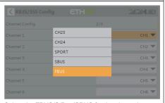
Select the FBUS/S.Port/SBUS for the channel ports.
