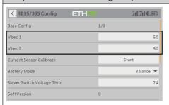
Dual BEC voltage outputs can be configured from 5-8.4V and supports device working with DC 2\*15A in this range.
