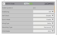
Note: The settings for Stable System 1 and 2 are independent, and both need to be calibrated when Self Check calibration is required.
