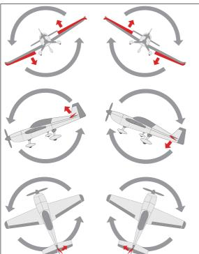
When the plane is rotated left or right (Roll), ailerons should have the correcting actions as illustrated.
