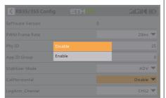
Changing the CaliHorizontal option from Disable to Enable can trigger horizontal plane calibration.
