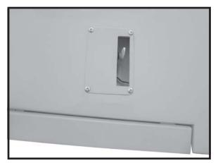
□ 2) Install the aileron servo mount into the wing, with the output shaft towards the leading edge of the wing.
