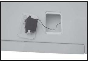
Attach a servo lead to the aileron servo. Attach the string to the servo lead and carefully thread it though the wing. Once you have thread the lead throught the wing, remove the string so it can use for the other servo lead. Tape the servo lead to the wing to prevent it from falling back into the wing.
