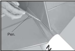
☐ 4) Remove the stabilizer. Using a modeling knife, remove the covering from below the lines you drew. Also remove the covering from the bottom edge of the stabilizer and the bottom and top edges of the filler block. Leave the covering in place on the sides of the filler block.
