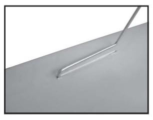
☐ 3) The landing gear wire is held in place using two nylon landing gear straps and four 3mm x 12mm wood screws.
