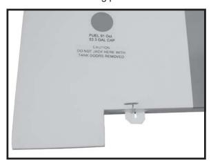
☐ 3) Slide the aileron on the wing panel until there is only a slight gap. The hinge is now centered on the wing panel and aileron. Remove the T-pins and snug the aileron against the wing panel. A gap of 1/64" or less should be maintained between the wing panel and aileron.
