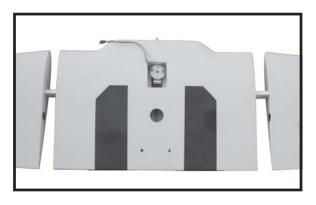
☐ 5) Apply masking tape at the wing join to hold the wing halves together securely.
