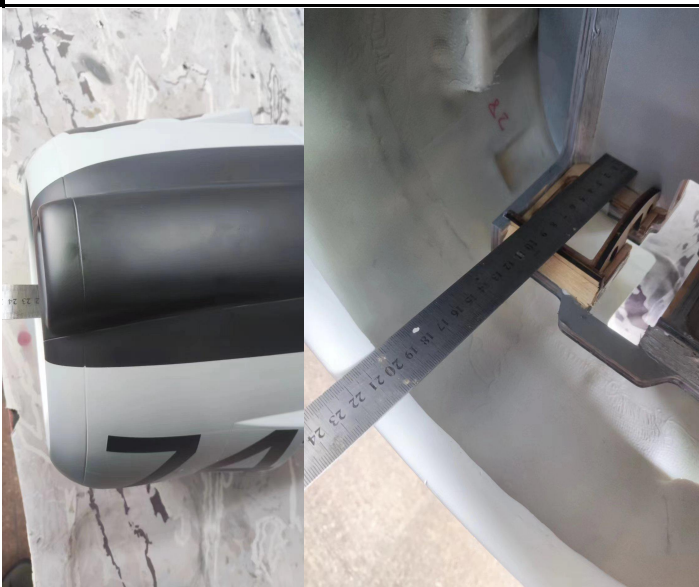
18 The widest sides of the cowling is 33.5 cm
