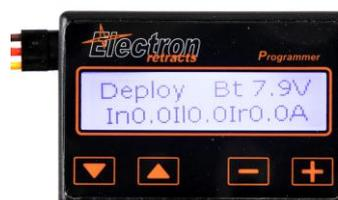
Pressing the arrow up button once, the screen will show the numeric values of the radio channels being input into the controller. From this screen you can verify that all connections and channels are working correctly.
