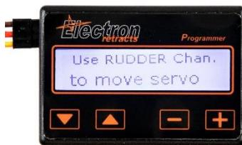
Moving on to the next screen pressing the up arrow, we start programming the output Out1.
