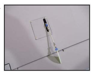
Set the aileron hatch in place and use a Phillips screw driver to install it with four wood screws.
