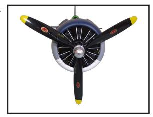
The propeller should not touch any part of the cowling. If it does, check and adjust engine mounting/cowl spacing as needed to where the propeller will not come in contact with the cowling.
