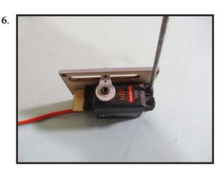
Apply 2-3 drops of thin C/A to each of the mounting aileron hatch mounting tabs in the wing. \*\*\*Allow the C/A to cure without using accelerator.\*\*\*
