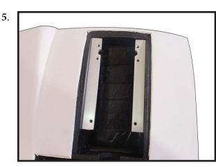
Install Main Retractable Landing Gear.
