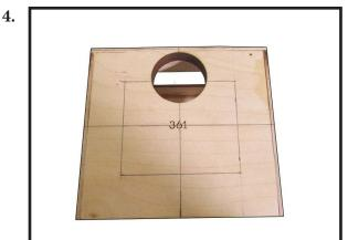
Attach the electric motor box to the firewall centered with the cross lines drawn on the electric motor box and firewall. Using M6x25mm to secure the motor box to the firewall. Please see pictures below.
