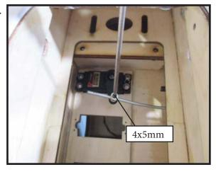
Move the throttle stick to the closed position and move the carburetor to closed.
