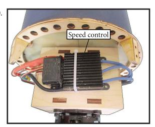
Attach the speed control to the side of the motor box using two-sided tape and tie wraps. Connect the appropriate leads from the speed control to the motor. Make sure the leads will not interfere with the operation of the motor.
