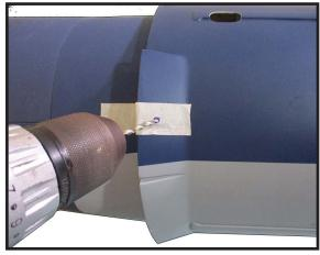
Install the muffler onto the engine and make the cutout in the cowl for muffler clearance. Connect the fuel and pressure lines to the carburetor, muffler and fuel filer valve. Secure the cowl to fuselage using the M3x10mm socket head screws. Putting a small length of silicone fuel tube under the head of the screw helps with vibration.
