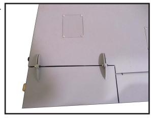
Set the flap control at the transmitter to the down flap position. Adjust the flap travel at the transmitter until it matches the control throws listed in this manual.
