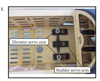
Install the rudder and elevator servo arms as shown above.
