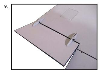
Once adjusted, make sure all clevis retainers are in position. Apply a drop of threadlock near the clevis, then tighten the nut against the clevis to keep the linkage from changing length inside the wing.
