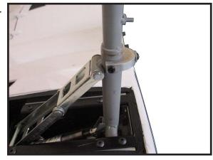
Install aluminum pieces into the landing gear struts as shown below.
