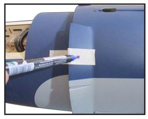
Use a drill and drill bit to drill the holes for the cowl mounting screws. Make sure the cowl position is correct before drilling each hole.
