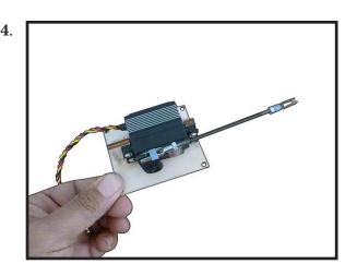
Attach the flap linkage to the control horn. Slide the clevis retainer over the forks of the clevis.
