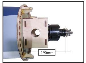
Then, use 5.2mm drill bit to enlarge the holes on the electric motor box.
