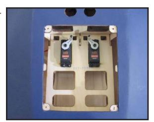
Install the gear door servo into the wing cover as shown below in these illustrated steps.
