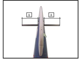
Use Epoxy to glue the Horizontal Stabilizer to the fuselage.
