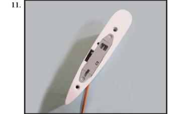
Install drop tank/bomb releases as shown.
