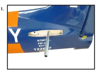
Use Epoxy Glue to glue the Horizontal Stabilizer to the fuselage.
