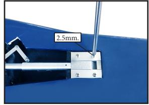
Install servo for Retractable landing gear.
