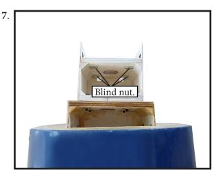
5) Attach the motor to the front of the electric motor box using four 4mm blind nut, four M4x20mm hex head bolts to secure the motor. Please see picture shown.
