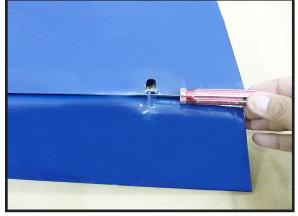
Attach the flap linkage to the control horn. Slide the clevis retainer over the forks of the clevis.
