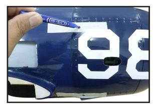
Use a drill and drill bit to drill the holes for the cowl mounting screws. Make sure the cowl position is correct before drilling each hole.
