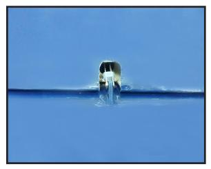
Attach the clevis to the flap servo arm.
