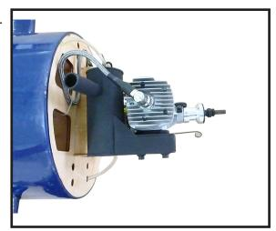
Move the throttle stick to the closed position and move the carburetor to closed. Use a 2.5mm hex wrench to tighten the screw that secures the throttle pushrod wire. Make sure to use threadlock on the screw so it does not vibrate loose.
