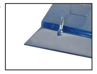
Once adjusted, make sure all clevis retainers are in position. Apply a drop of threadlock near the clevis, then tighten the nut against the clevis to keep the linkage from changing length inside the wing.
