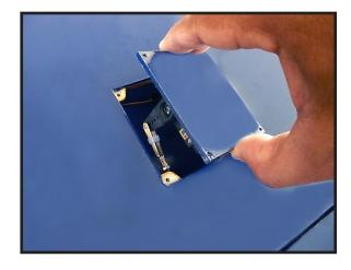
Route the servo lead for the flap servo out at the root of the wing. Connect the flap servo to the radio system. With the radio system on, place the flap servo into position.
