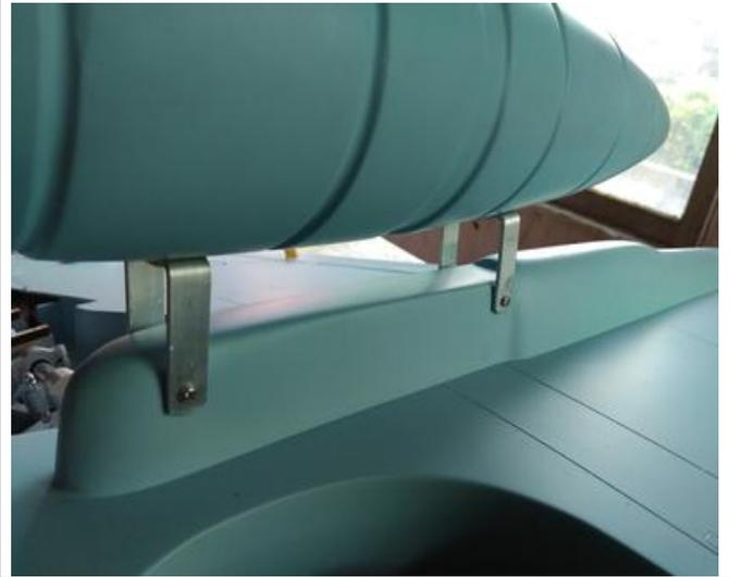
29. Assemble the engine to the engine mount.
