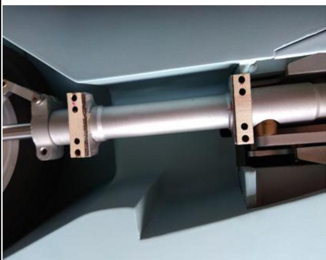
**24. Assemble the wheel cover to the oleo struts with screws.**
