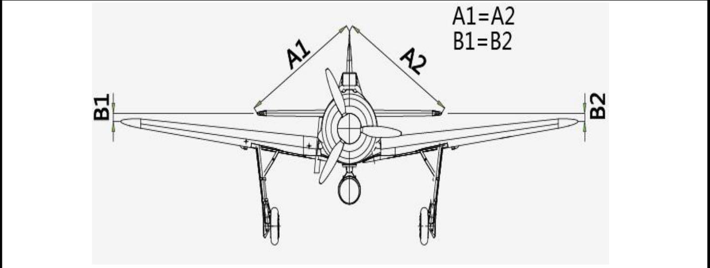
40. C.G: Never fly before checking the CG's required position. Never fly the model without well balancing.
