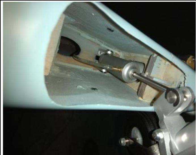
18. Fix the air cylinder to the tail fuselage.
