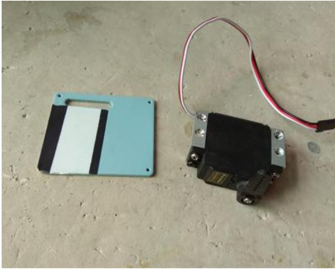
7. Assemble the servos to the servo trays.
