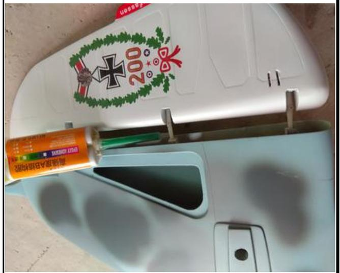
16. Picture of the rudder install ready, make sure it can rotate smoothly.
