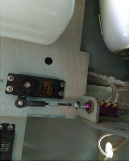
27. Assemble the air tube to the air tank.
