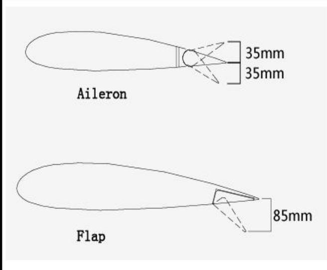
38. Adjust the travel of each control surface to the values in the diagrams. These values fit general flight capabilities. Readjust according to your needs and flight level.
