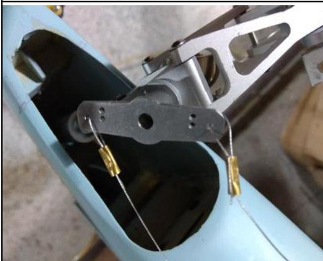
20. Drill a small hole to appropriate position in the fuselage, connect the rudder to the servo in the fuselage via steel wire.
