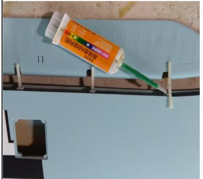
4. Epoxy the aileron to the wing, Keep some space between the trailing edge and the aileron to make sure it can rotate smoothly.
