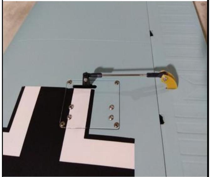
10. Connect the fiber horns in the flap to the servo arms with the linkage and lock each side with screws and nut.
