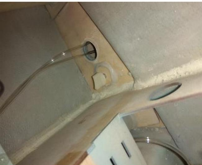
33. Fixing the stab with screws from bottom of the stab.
