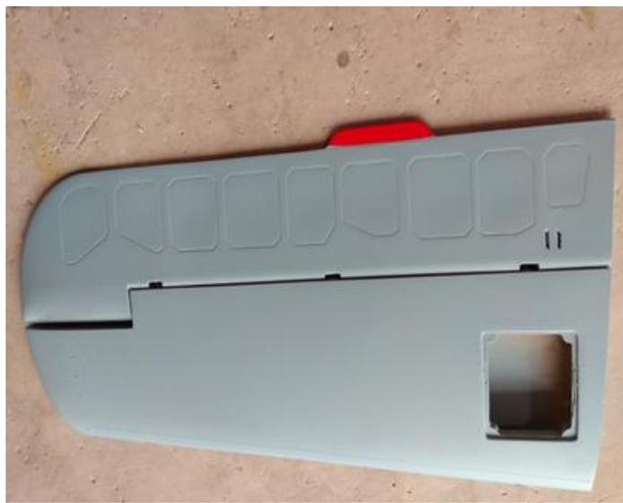
13. Apply AB glue to the slots in the elevator and assemble the horns into them.
