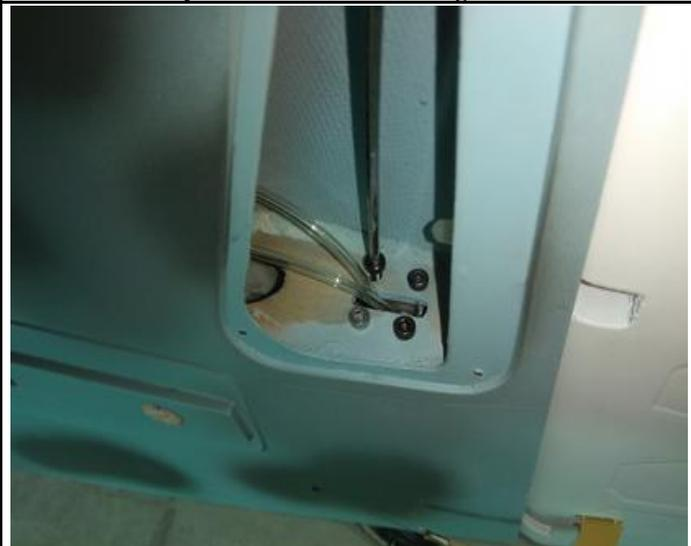
19. Connect the arm of the tail landing gear with steel wire.
