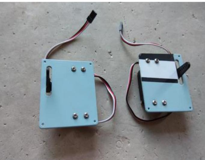
9. Connect the fiber horns in the aileron to the servo arms with the linkage and lock each side with screws and nut.
