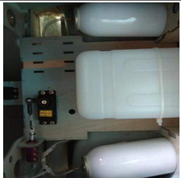
26. Assemble the air tubes to the switch valve.
