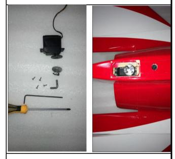
10. Install the servo cover to the tail fuselage with screws as pictures below .
