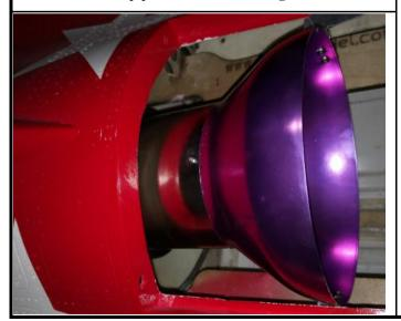
**18.** Put the fiber exhaust into the tail fuselage and lock it with screws .
