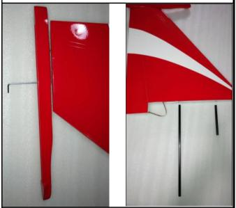
5. Assemble the wing to the fuselage through the carbon fiber bar, allow the servo lines go inside the fuselage, secure the wing with the screws from the holes in bottom
