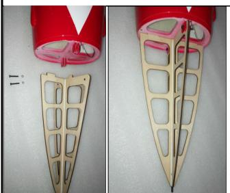
21.Put the plane nose to the fuselageuntil they fit very well, assemble the antena to the plane nose throught the threaded rod .
