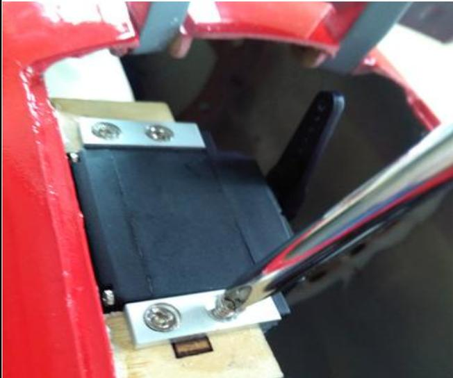
30. Connect the belly speed brake to servo arms with the linkage and locked each side with screws.
