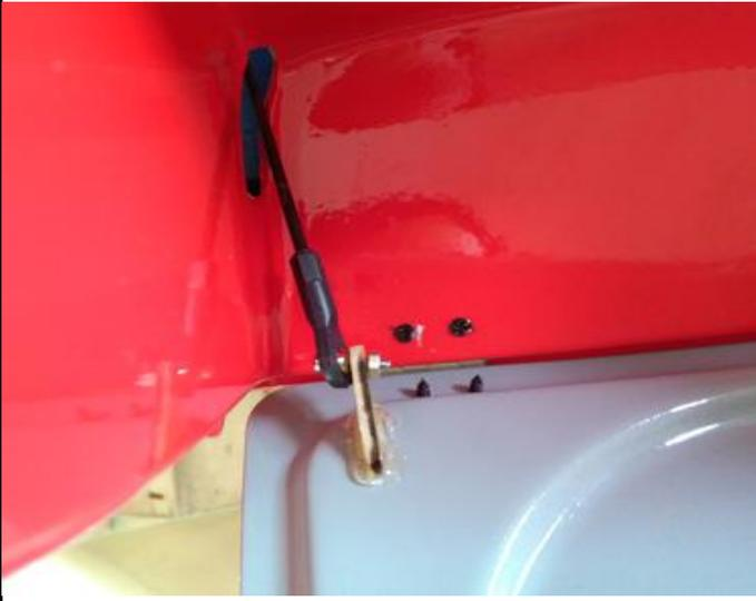
40. Connect the linkage to the fiber horn with screws and locknuts.
