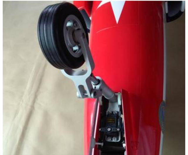
**53. Connect the hatch hinge to the clevis on the Alu sash with screw.**
