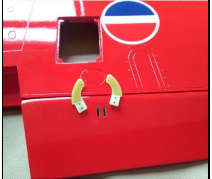
4. Fix the fiber horns to the slots in the aileron with epoxy glue.
