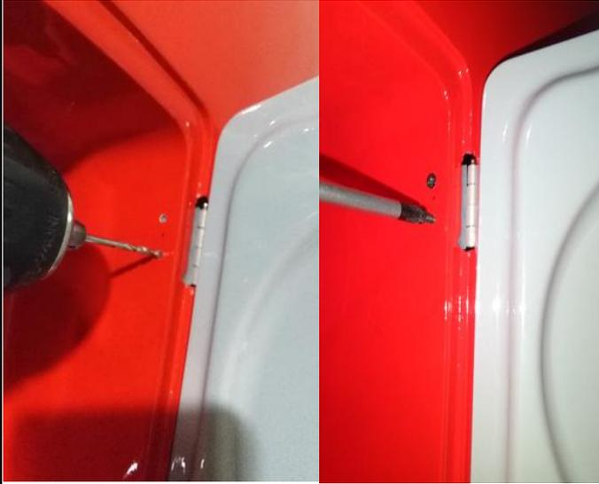
34. Drill holes to appropriate position in the wheel doors and lock the wheel doors with screws.
