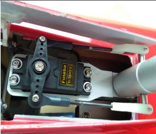
**52. Fix the nose retract to the fuselage with screws.**
