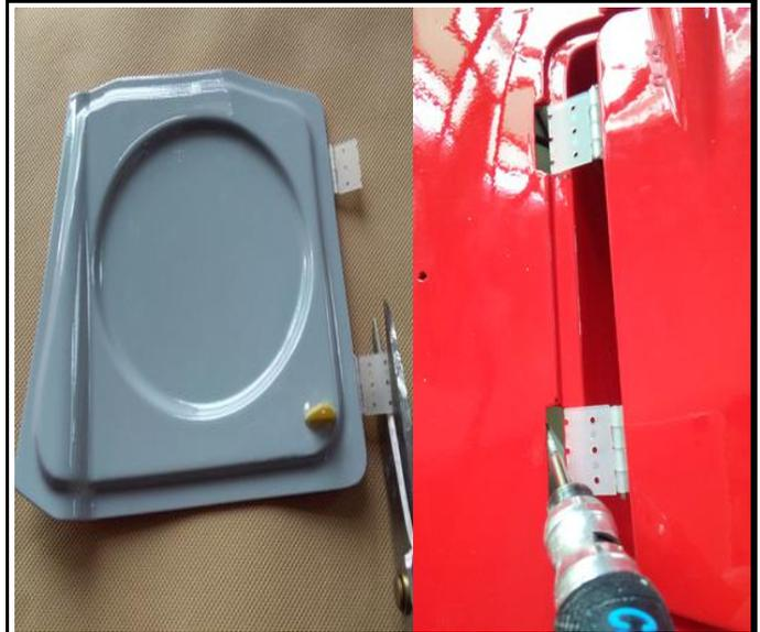
33. Drill holes to appropriate position in the fuselage and lock the wheel doors with screws.
