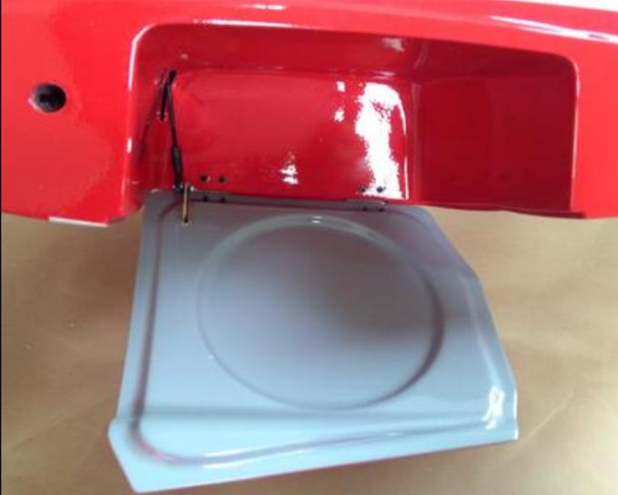
41. Connect the linkage to the servos for wheel doors.
