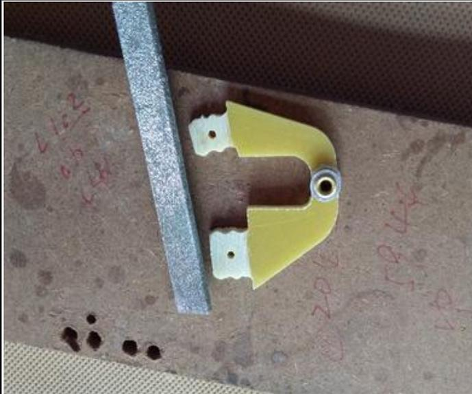
3. Fix the fiber horns to the slots in the aileron with epoxy glue.
