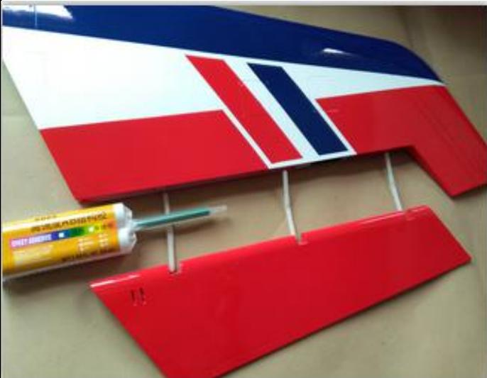
19. Assemble the rudder to the vertical fin and make sure it can move freely.
