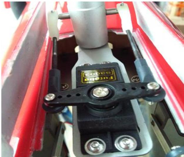
**51. Put the retract to the appropriate position from inner fuselage.**
