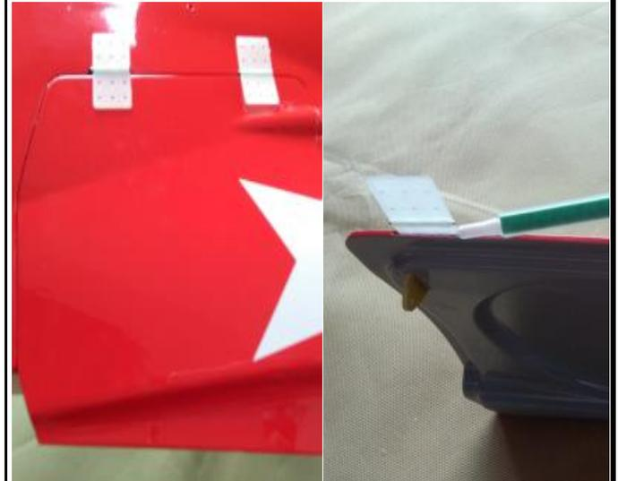
32. Cut surplus the pinned hinges, put the wheel doors to the fuselage via the opened slots.
